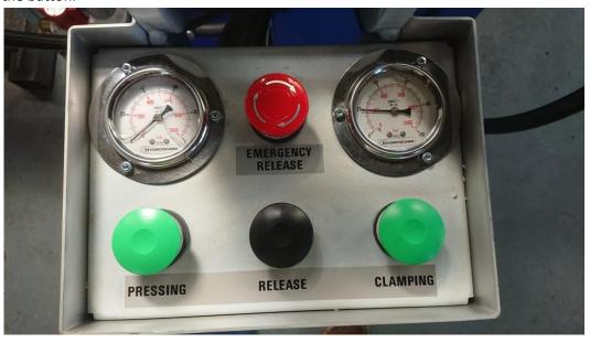
10. "EMERGENCY RELEASE" will release the clamping cylinders. This will happen even if there is no air supply because of a small air reservoir in the system.
