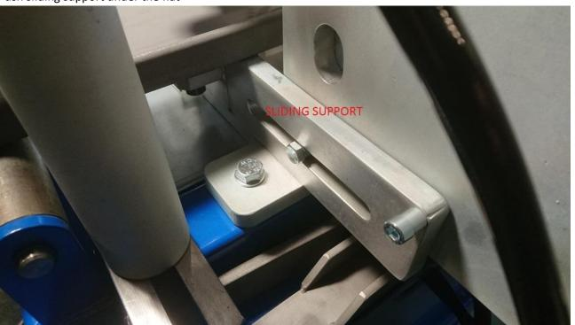
6. Place the hold-down support on the end of the bulb flat. This is to prevent the bent bulb from rising up during and after the press. Supports are specific for each size of bulb flats and are stamped accordingly.
