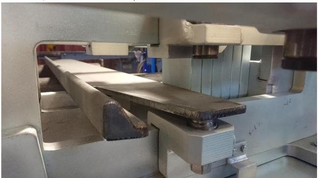
3. Place necessary amount of shims behind the bulb flat. E.g. HP 160 = 6 shims.
